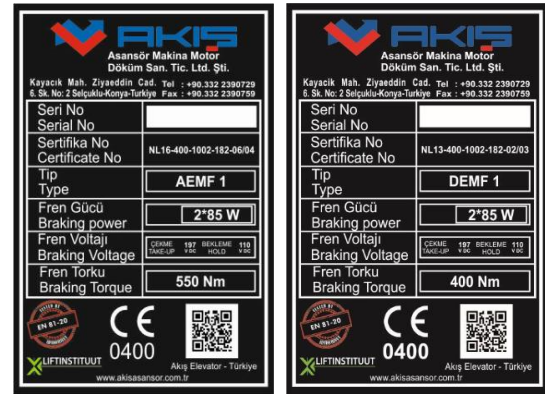
Figure 5. Example of data plate with nominal characteristics of brake.
